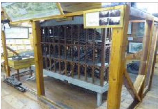
**Model of Kennedy Tailing Wheel #4 - the model is built at a scale of 1 inch equals 1 foot**
