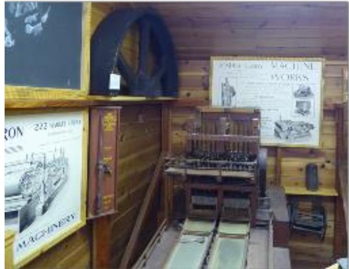
***Model of the North Star Mine Stamp Mill - the model is built at a scale of 1 inch equals 1 foot***
